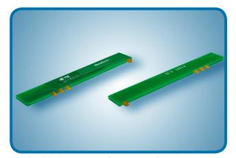
Embedded Antennas for LTE applications
